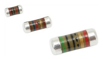
MMU 0102 HF, MMA 0204 HF, and MMB 0207 HF specialty thin film MELF resistors for RF applications are the perfect choice in high frequency circuit designs where the impedance change due to the parasitic inductance of regular and professional resistors can not be accepted. Typical applications are in the fields of telecommunication equipment and industrial electronics.
